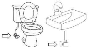
The Agua-Scope sensor head must be connected
