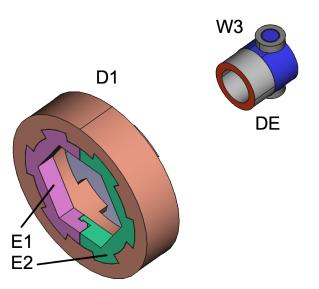
The valves from this company have a unique design. You must insert the split ring (E1+E2) into the 24 mm spacer ring (D1) instead of using one of the adapters A1 ... A4. A small additional spacer ring (DE) is placed directly under the ball bearing seat to fix the valve's grease chamber.
