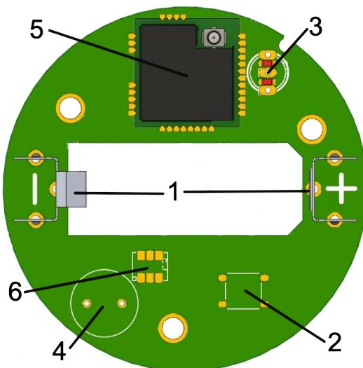
After inserting the battery, the LEDs will blink red/green. This indicates an attempt to JOIN the LoRaWAN network. Success is indicated by 3 \* green blinks, failure is indicated by 3 \* red blinks. Pressing the button will always force a rejoin if the
